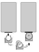
\*When purchased the remote control has a battery installed with a plastic insert to prevent battery discharge. Remove the plastic insert before attempting to use the remote.
